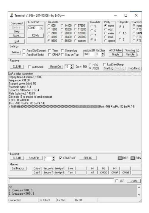
Figure 4: Serial print data from LoRa echo Transmitter.
