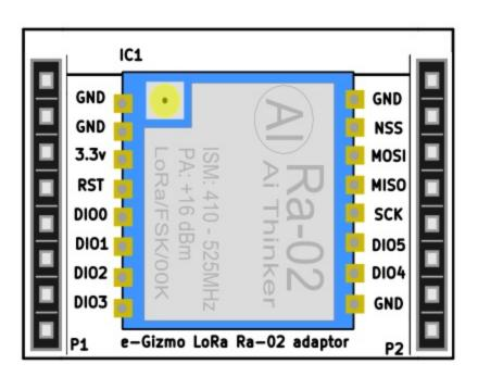
Figure 1. Major Part of LORA RA-02 module with adaptor.
