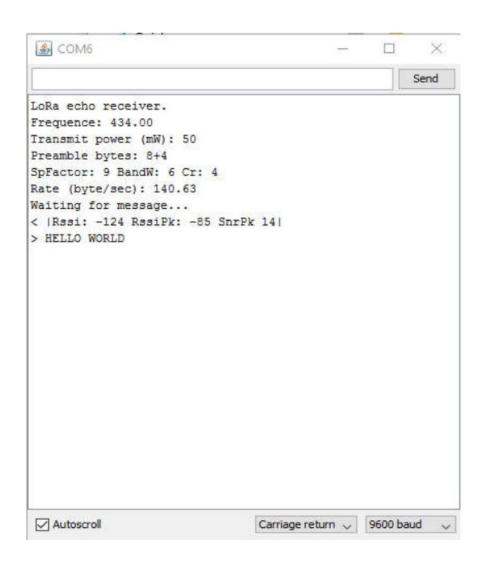
Figure 5: Serial print data from LoRa echo Receiver.
